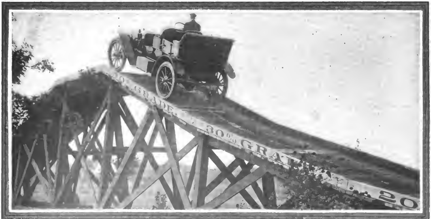
Fig. 14 Special grade constructed to try out Rambler automobiles before delivery affording great advantage
